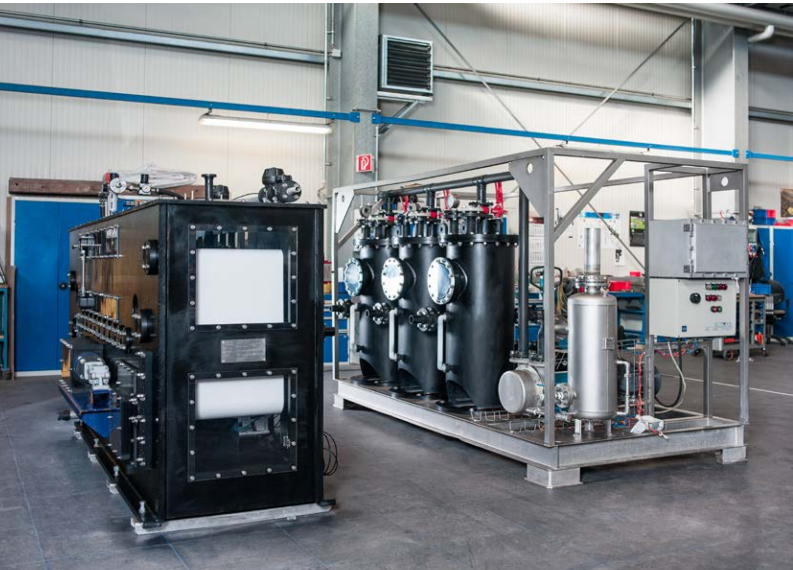
Pilot indexing belt filter plant in closed hood for tests
