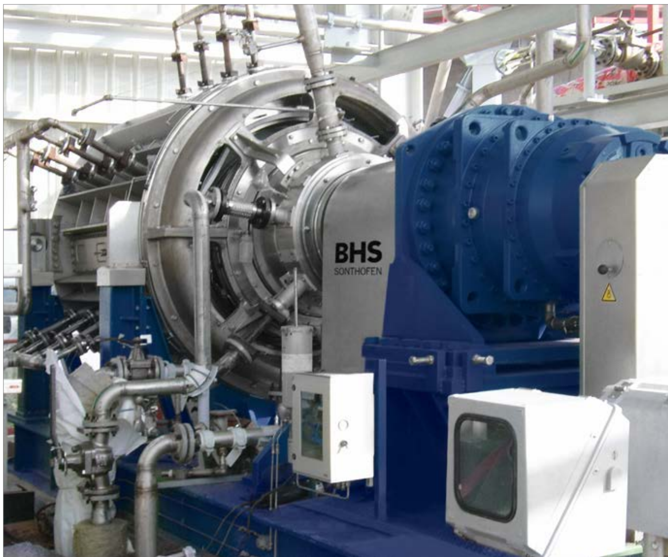
RPF B16 rotary pressure filter for the production of plastic intermediates
