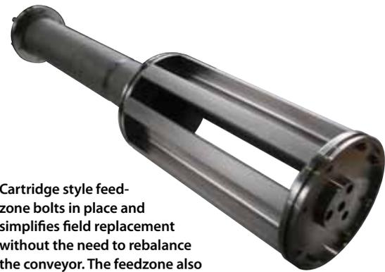
**Cartridge style feed-zone bolts in place and simplifies field replacement without the need to rebalance the conveyor. The feedzone also offers integrated wear inserts with B&P's new wear coating to increase longevity.**
