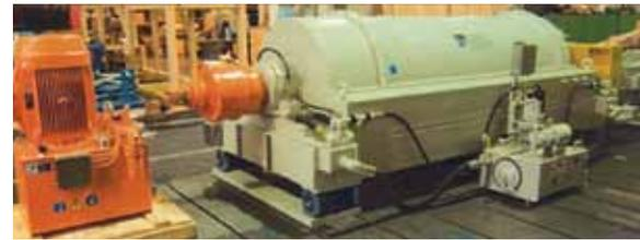
**360° solids discharge ports maximize the discharge area. Also includes replaceable wear liners with B&P's new wear coating to increase longevity.**
