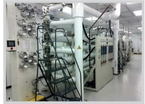
The scientific line size is ideal for precursor development and validation, as material property data can be obtained from small samples. It does not require cooling water of natural gas and uses low emissions so that volatiles can be safely vented to outdoors without abatement equipment.
