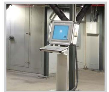
Harper's advanced operator-interface enables simple control of temperature, alarm management, sensor calibration, program recipe storage and retrieval, archiving of data and interface to central control systems of the thermal units, as well as advanced functions such as remote monitoring and proactive predictive maintenance.
